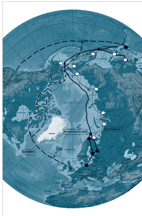
Figure IV.4 Trans-Arctic communication cable projects
